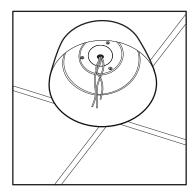
Figure 3. Installing the Surface Mount Back Box
